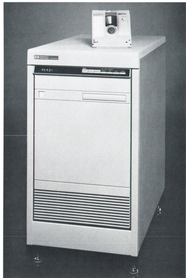
Fig. 1. The HP Series 6300 Model 20GB/A rewritable optical disk library system stores up to 20.8 Gbytes of data on 32 optical disks. An autochanger automatically selects the correct disk and inserts it into one of two internal drives.
